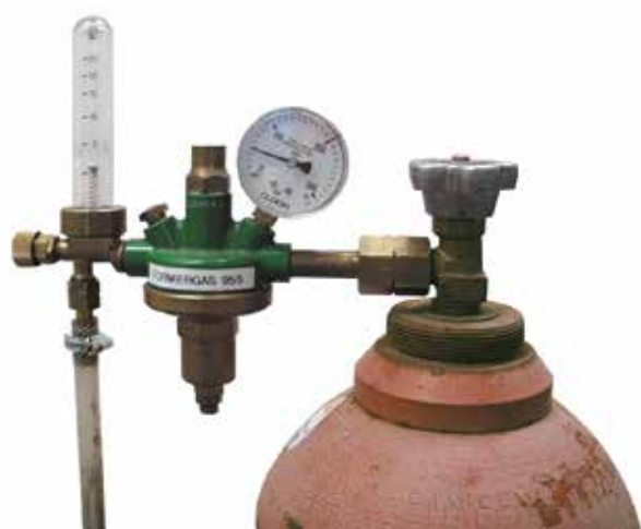
Pressure reducing valve with assembled flow meter
