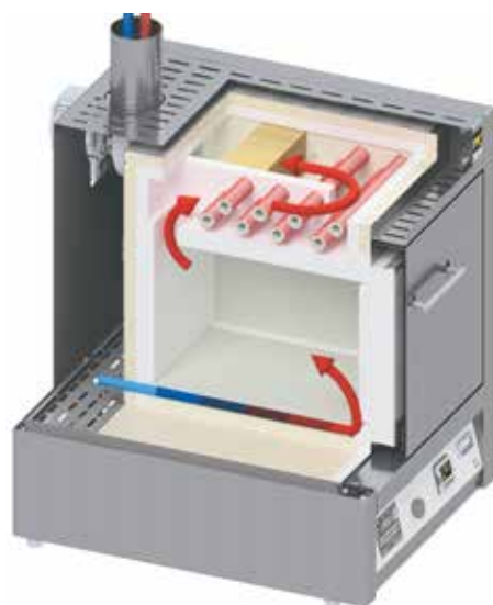
Schematic presentation of air circulation in ashing furnace L 24/11 BO
