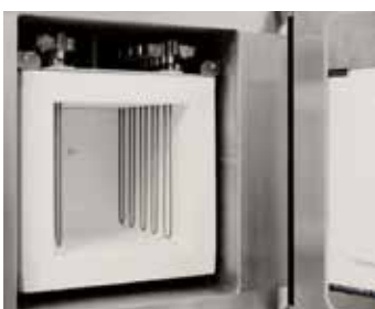
Molybdenumdisilicide heater and fiber insulation
