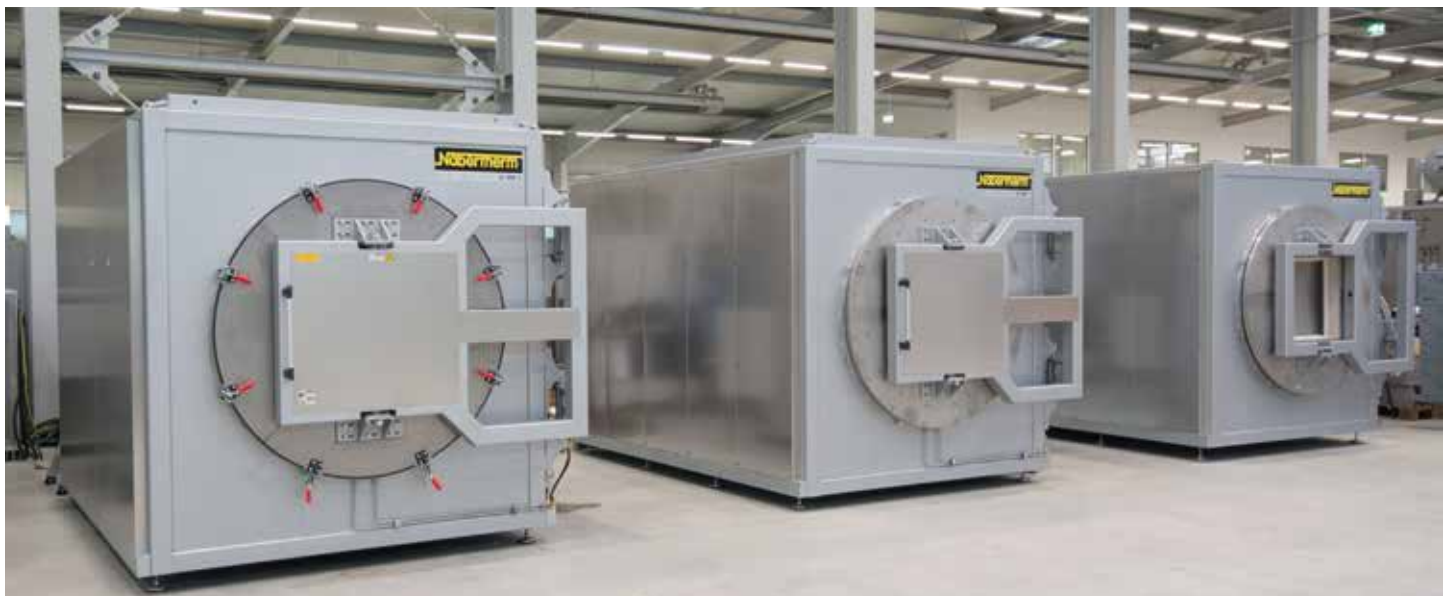
Hot-wall retort furnaces NR 1000/11 in production
