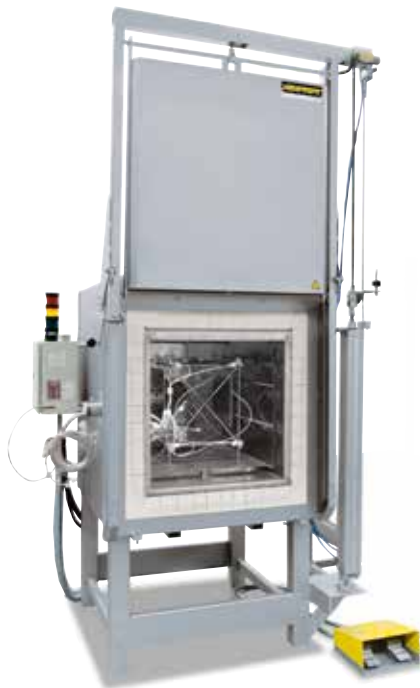
Holding frame for measurement of temperature uniformity
