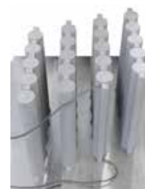
Titanium rods after heat treatment in NR 50/11 in argon atmosphere
